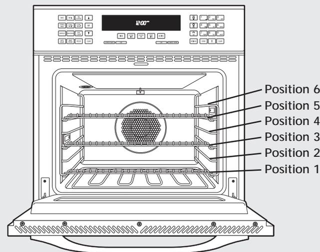
All ovens have six rack positions. Position 6 is the farthest from the oven bottom. Position 1 is the closest to the oven bottom. The racks can be easily removed and arranged at various levels. For best results with conventional baking, do not use more than one rack at a time. It is also recommended, when using two racks, to bake with the racks in positions 2 and 4 or positions 3 and 5.
